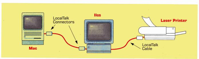
Figure 1. Snap together a simple two-computer/one-printer AppleTalk network in 15 minutes.
